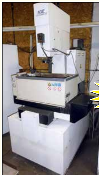
AGIE Cut Classic Wire EDM , Mdl. Classic 2S, AWF and submerged, 20' x 21' platen, X=13.77", Y=9.84", Z=10", 29.5" x 21.6" x 9.8" max. work piece, 992-lb. max. table cap., 28"/min., SN 501, 2004.
