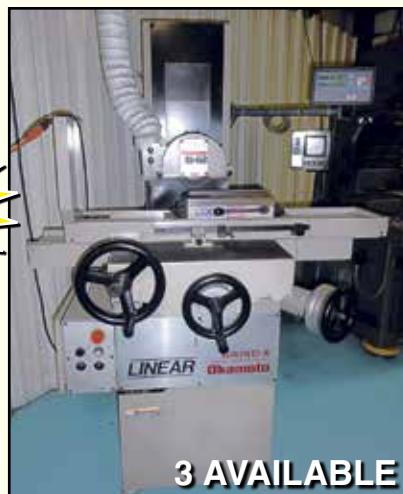
(3) OKAMOTO Surface Grinders , Mdl. 6-12/14, 6" x 14" mag. chuck, 8" wheel, 15" travel, 1.5 HP, w/2-axis DRO, SN's 2746U (1994), 2674U (1994), 2434U.
