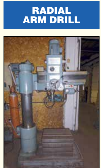
LINCOLN Radial Arm Drill, Mdl. 820, 8" column, 36" arm, 24" x 18" box table, SN 12777, 1995.
