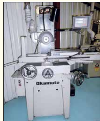
OKAMOTO Surface Grinder , Mdl. 6-18, 6" x 18" mag. chuck, 8" wheel, 14" travel, 2 HP, w/2-axis DRO, SN 4565, 1993.
