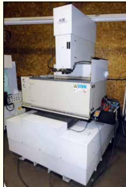
AGIE Sinker EDM , Mdl. Elox Mondo 50, 29.5" x 21.65" work table, X=19.6", Y=13.7", Z=13.7", 33.8" x 25.6" x 12.4" max. work piece, 1,100-lb. max. table cap., 37"/min., SN MON50-003116, 1998.
