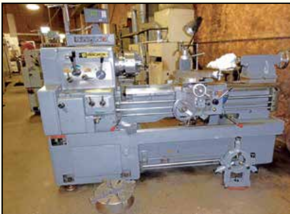
< HWACHEON Gap Bed Lathes , Mdl. 18-40, 18" swing, 40" centers, 24" swing in gap, 2-axis DRO, 2" spindle bore, 12" 4-jaw chuck, TS, SR, SN 222266, 1993.
