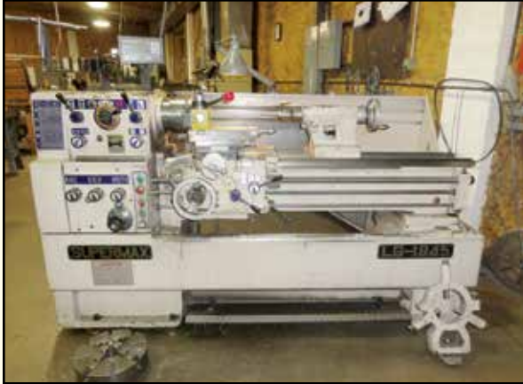
< SUPERMAX Gap Bed Lathe , Mdl. LG-1845, 18" swing, 50" centers, 24" swing in gap, 12" swing over CS, 2-axis DRO, 2.25" spindle bore, 12" 4-jaw chuck, TS, SR, SN R8603-012, 1997.
