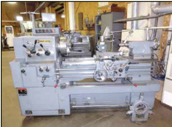
< HWACHEON Gap Bed Lathes , Mdl. 18-40, 18" swing, 40" centers, 24" swing in gap, 2-axis DRO, 2" spindle bore, 12" 4-jaw chuck, TS, SR, SN 224862, 1997.
