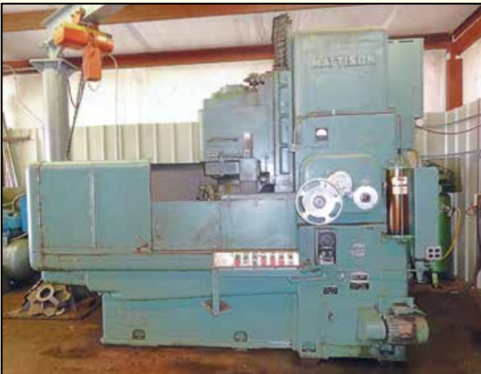
MATTSON Rotary Surface Grinder, #24-12, 36" mag. chuck, 40 HP, 1/2" chuck life, SN 24601.
