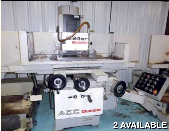
(2) OKAMOTO Surface Grinders, Mdl. ACC 12-24ST, 11.75" x 23.5" mag. chuck, 12" wheel, 29.5" travel, 5 HP, SN's 83684 (2003), 83388 (1998).
