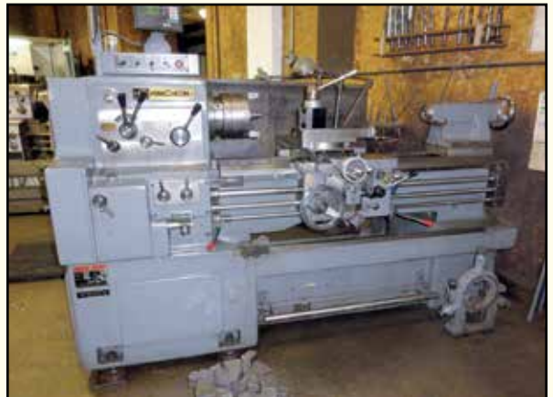
< HWACHEON Gap Bed Lathes , Mdl. 18-40, 18" swing, 40" centers, 24" swing in gap, 2-axis DRO, 2" spindle bore, 12" 4-jaw chuck, TS, SR, SN 224862, 1997.
