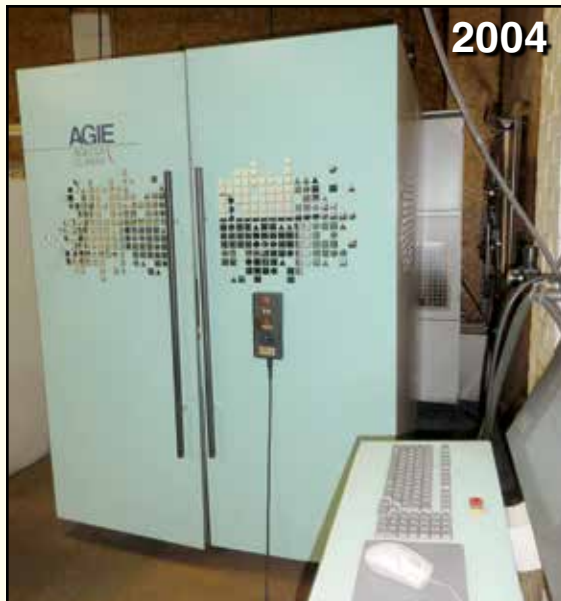
AGIE Cut Classic Wire EDM , Mdl. Classic 2S, AWF and submerged, 20' x 21' platen, X=13.77", Y=9.84", Z=10", 29.5" x 21.6" x 9.8" max. work piece, 992-lb. max. table cap., 28"/min., SN 501, 2004.
