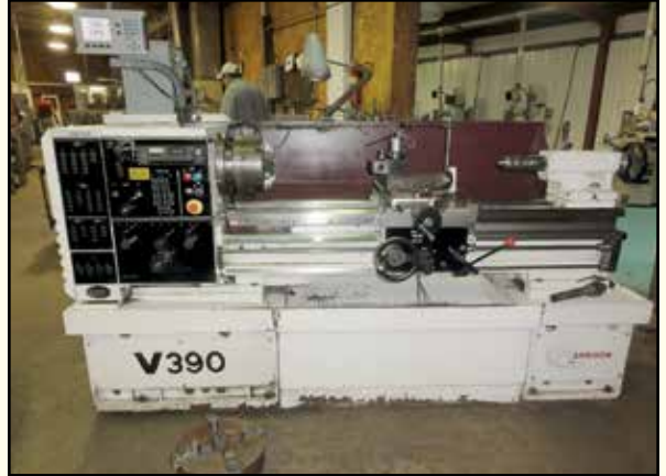
< SUPERMAX Gap Bed Lathe , Mdl. LG-1845, 18" swing, 50" centers, 24" swing in gap, 12" swing over CS, 2-axis DRO, 2.25" spindle bore, 12" 4-jaw chuck, TS, SR, SN R8603-012, 1997.
