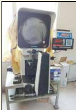
DELTRONIC Optical Comparator, Mdl. MPC-5, 14" w/Deltonics MPC5 2-axis DRO.
