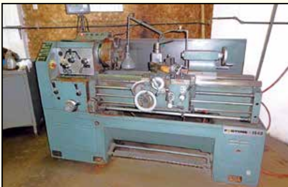
< FORTUNE 1640 Gap Bed Lathe , Mdl. 1640, 16" swing, 40" centers, 22" swing in gap, 9.4" swing over CS, 2-axis DRO, 2" spindle bore, 12" 4-jaw chuck, TS, SR, SN 564744.
