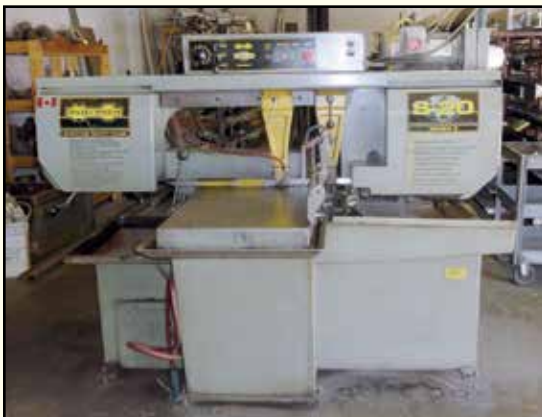
HYD-MECH Horizontal Miter Bandsaw, Mdl. S-20, Series II, 13" x 18" cap. @ 90 deg., 3 HP, 1" blade, SN 60490578.
