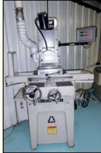
OKAMOTO Surface Grinder, Mdl. PFG 612, 6" x 12" mag. chuck, 8" wheel, 14" travel, 1.5 HP, w/2-axis DRO, SN 62066, 2000.
