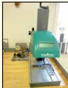
PROPEN Engraver , Mdl. P3000N PN, 4" x 4" marking zone, 12" max. material thickness, SN P3000-00-03-01436, 2000.
