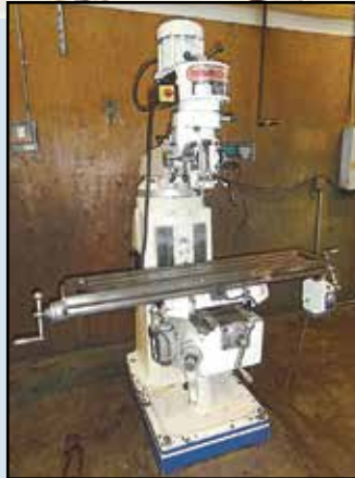
(2) BIRMINGHAM Mills , Mdl. X6323A, 9" x 48" tables, 2-axis DRO, PF@X, VS, SN 054671, SN 054568, 2005.
