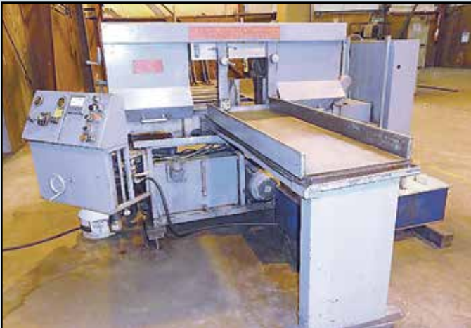
MEDALIST PEERLESS Horizontal Saw , 1400 Series, 13.5" x 21" cap., SN 1400-139-81.
