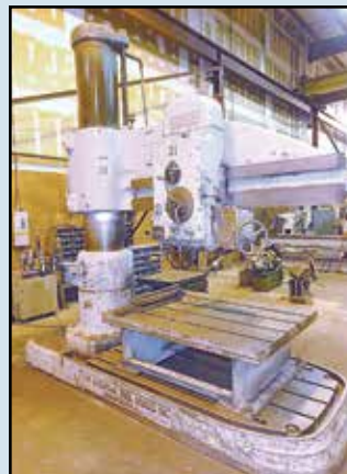
< AMERICAN Hole Wizard Radial Drill , 17" column x 6" arm, 44" x 60" box table, 30" x 20" table, #5 Morse taper, 1,200 max. RPM.
