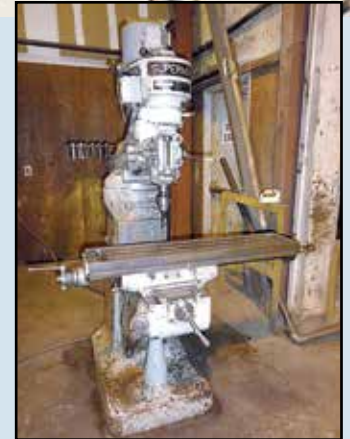
SUPERMAX Vertical Mill , 9" x 43" table, SN 81-047140.
