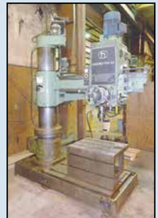
< AMERICAN Hole Wizard Radial Drill , 17" column x 6" arm, 44" x 60" box table, 30" x 20" table, #5 Morse taper, 1,200 max. RPM.
