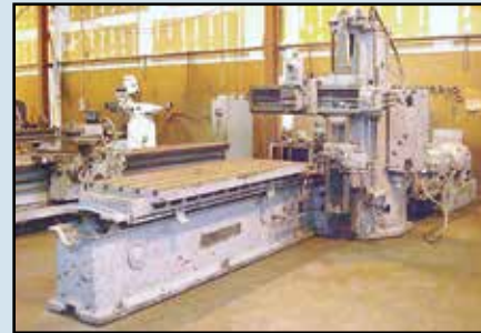
(2) BIRMINGHAM Mills , Mdl. X6323A, 9" x 48" tables, 2-axis DRO, PF@X, VS, SN 054671, SN 054568, 2005.
