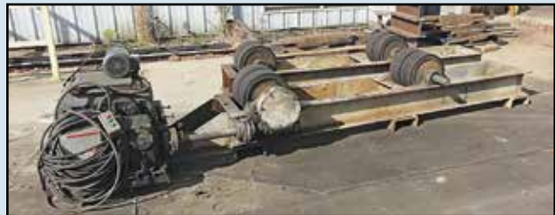
RANSOME Power Turning Rolls , 50-ton cap., SN 8678.
