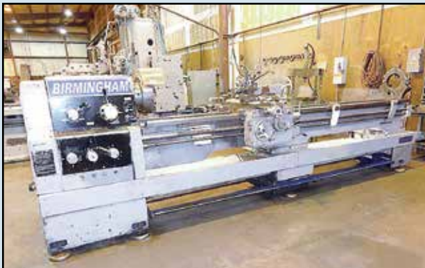
< BIRMINGHAM Gap Bed Lathe , Mdl. DL-18120, 18" max swing, 27.5" in gap, 120" DBC, 3-3/16" spindle bore, 16-1,600 RPM, 10 HP, taper attach., TS, SR, 12" 4-jaw chuck, SN F327.
