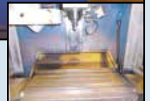
VIPER VMC , Mdl. 850-P, X=32", Y=20", Z=24.8", 32" x 18" table, Cat 40 tooling, 20-ATC, 10 HP, 8,000 RPM, w/Meldas M500 Series control, SN 912804-004, 1997.
