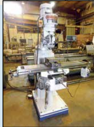
(2) BIRMINGHAM Mills , Mdl. X6323A, 9" x 48" tables, 2-axis DRO, PF@X, VS, SN 054671, SN 054568, 2005.
