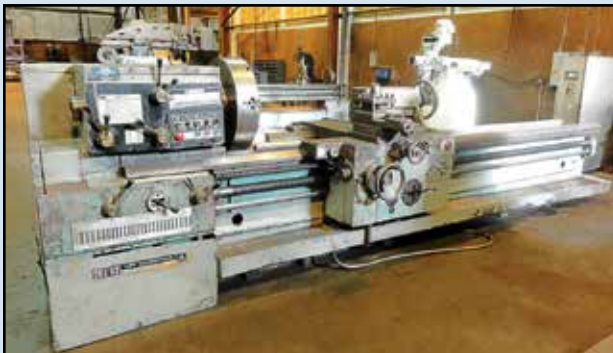
TOS Engine Lathe , Mdl. SUS63, 25" swing, 120" DBC, 3.25" spindle bore, 9-1120 RPM, 30 HP, taper attach., TS, 24" 4-jaw chuck, SN 0440534.
