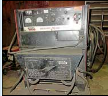
(5) LINCOLN DC600 Wire Welders.
