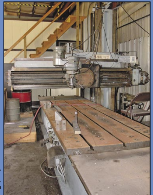
> LIBERTY Horizontal Planer Mill , 10' x 58" table, 44" travel, 24' bed travel, 94" horizontal head travel, 2-axis DRO, s/n J-01050281280, Bridgeport-style converted head, variable speed.
