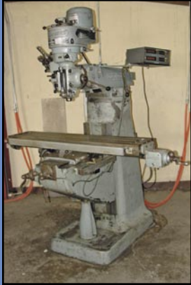
BRIDGEPORT 9" x 42" Vertical Mill, SP, w/Mitutoyo 2-axis DRO, s/n 80167.
