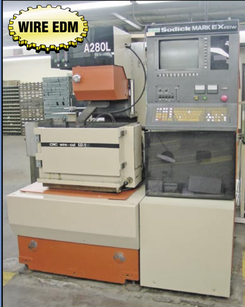
SODICK Mdl. A280L Wire EDM , Mark EXEDW controls, 20" x 30" tank capacity, travels 12" x 8" x 6.7", 1990.
