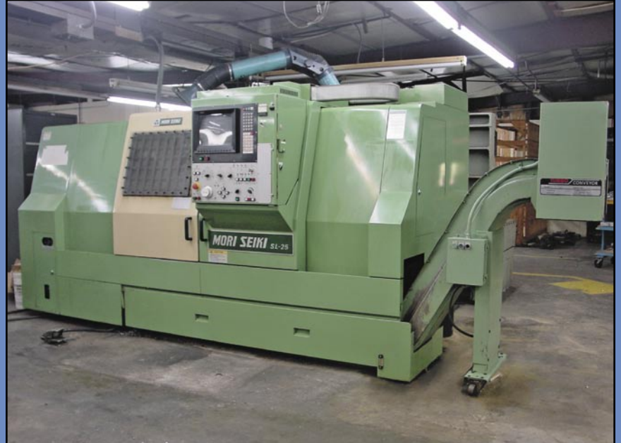
MORI SEIKI Mdl. SL25/500 Lathe , 20.5" x 24.6" bed, X=6.3", Y=24.6", 20 hp., w/chip conveyor, 13.7" cross slide, 40" centers, 20 hp., 6-station turret, programmable tailstock, MY-T3 control, auto. cutting time 5,248 hrs., power on time 31,024 hrs., 1987.
