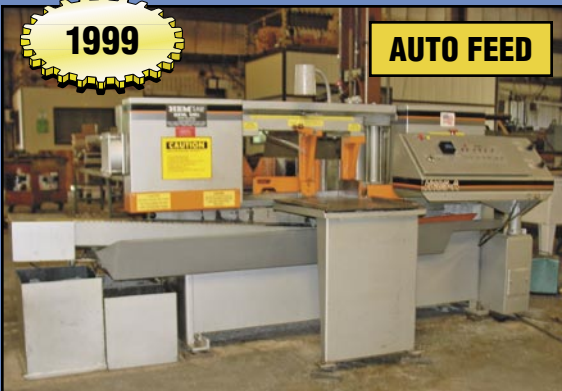
HE&M Mdl. H105-A Automatic Horizontal Band Saw , 14" x 16" cap., chip auger, power blade tension, auto feed, w/20' runout roller conveyor, s/n 653499, 1999.
