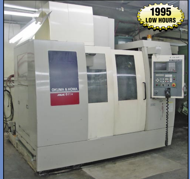
OKUMA & HOWA Mdl. Millac511 Vertical Machining Center , travel 40" x 20" x 20.47", Fanuc 18M controls, 40 taper, 20 ATC, 10,000 RPM, 25 hp., 4th axis compatible, s/n 5075, cutting time 1,436 hrs., power on time 20,818 hrs., 1995.
