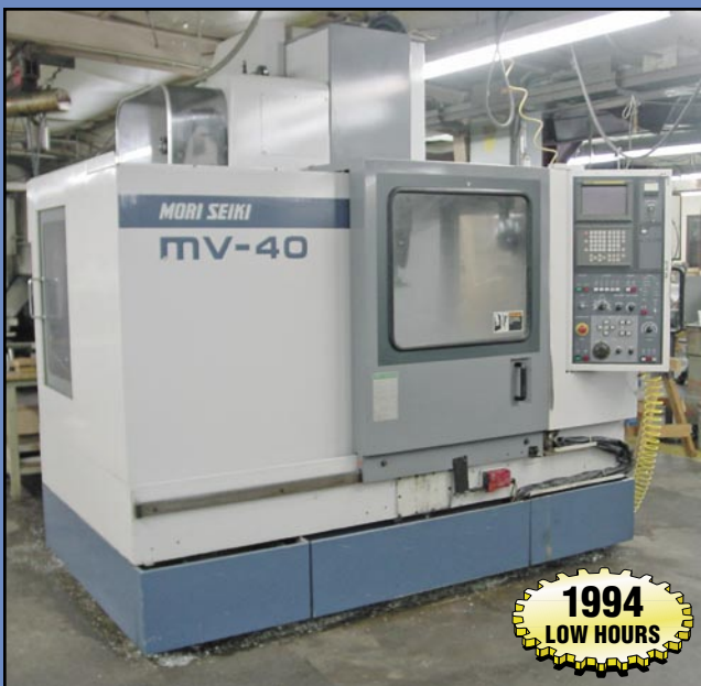
MORI SEIKI Mdl. MV40B Vertical Machining Center , travel 31.4" x 16.1" x 20", 40 taper, MF-M6 controls, 20 ATC, 15 hp., 4th axis compatible, s/n 003499, cutting time 817 hrs., power on time 26,725 hrs., 1994.
