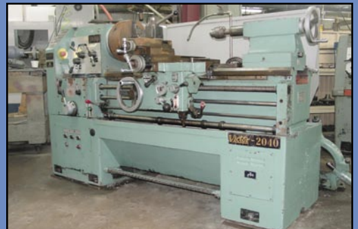
VICTOR Mdl. 2040 Engine Lathe, 20" x 40" threading, 3.25" spindle bore, 12" 3-jaw chuck, steady rest, 5 hp., s/n 760192.
