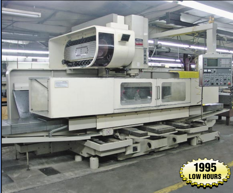
OKUMA & HOWA Mdl. Millac65V Vertical Machining Center , travel 22.83" x 25.59" x 78.74", Fanuc 16M controls, 50 taper, 30 ATC, chip conveyor, 25 hp., 4th axis compatible, s/n 66884, cutting time 1,629.46 hrs., power on time 20,892 hrs., 1995.
