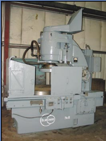
BLANCHARD Mdl. 18 Rotary Surface Grinder, 42" magnetic chuck, 50 hp., s/n 8758.
