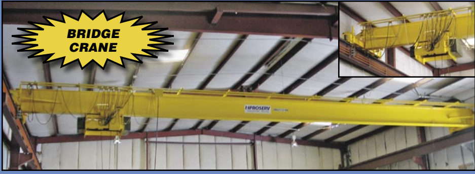
PROSERVE Bridge Crane , 60' span, single girder, top running, w/Shepard Niles 10-ton underslung hoist, 110' of rail, pendulum controls.
