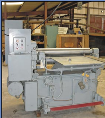
NIAGARA Mdl. 5-36 Plate Roll , 36" x 3/16" cap., 30" x 20" work table, s/n 57221.
