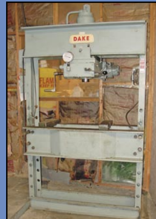
DAKE Mdl. 5-076 Hydraulic H-Frame Press , 75-ton cap., s/n 162688.
