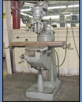
BRIDGEPORT Vertical 9" x 42" Mill, VS, 2-axis DRO, power feed at X, s/n 197984, Bridgeport shaping attachment, s/n E6447.
