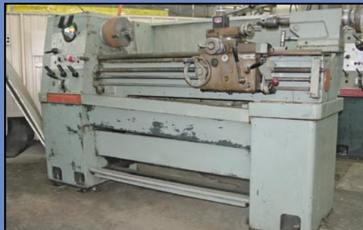
CLAUSING COLCHESTER Engine Lathe, 13" x 40", threading, collet closer, tailstock, 8" 3-jaw chuck, 10 hp., s/n 5/0014/04613.
