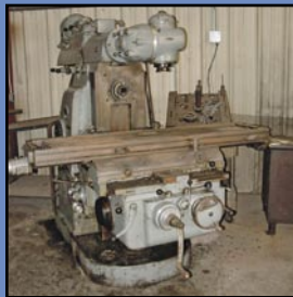
CINCINNATI No. 3 Horizontal Mill, w/vertical head attachment, 16" x 65" table, 7.5 hp., s/n 4J3T1Z-2.
