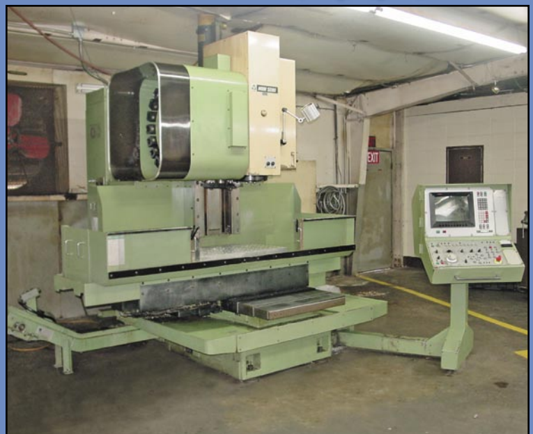
MORI-SEIKI Mdl. 45/40 Vertical Machining Center , travel 23.6" x 18.1" x 20.1", Fanuc MRC 1 controls, 40 taper, chip conveyor, 20 ATC, 15 hp., 1984.
