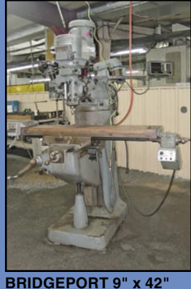
BRIDGEPORT 9" x 42" Vertical Mill, VS, 2-axis DRO, power feed at X, s/n 214811.
