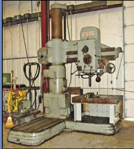
AMERICAN Hole Wizard C1-32-20-02 Radial Arm Drill , double pedestal base, 33" x 48" shop made box table, 13" column, 4' arm, 5 hp.
