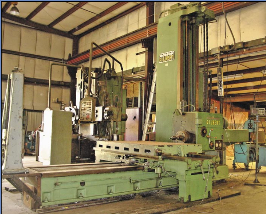
> LIBERTY Horizontal Planer Mill , 10' x 58" table, 44" travel, 24' bed travel, 94" horizontal head travel, 2-axis DRO, s/n J-01050281280, Bridgeport-style converted head, variable speed.
