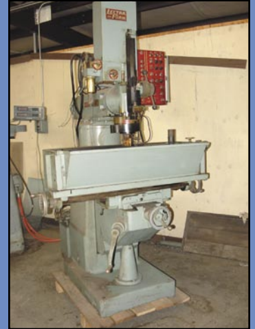
EX-CELL-O CORP. Elox Mdl. 242 EDM , 19" x 38" tank, 30" x 7' work surface.
