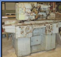
CINCINNATI Mdl. 1024 Universal Grinder, 10" x 24" x 13" wheel cap., w/ID attachment, 5 hp.
