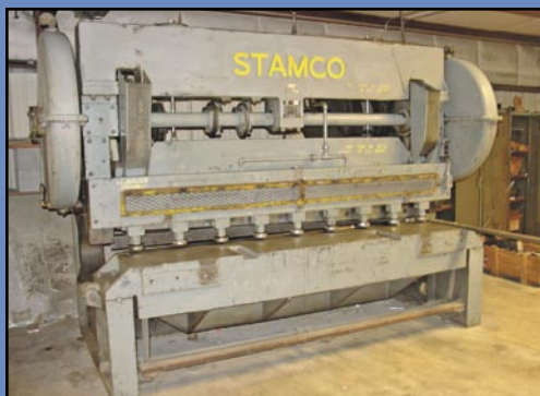
STAMCO Mechanical Shear , 8' x 3/16" cap., 4' squaring arm, ROBG, s/n L7651.
