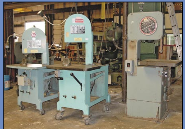
DoALL Mdl. 16-M Vertical Band Saw , 24" x 24" x 10", s/n 13459187; Roll-In Band Saw , 30.5" x 18" x 15"; Roll-In Band Saw , 18.5" x 19.5" x 10".
