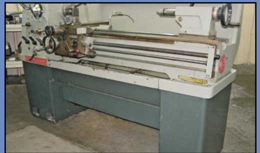
CLAUSING COLCHESTER Engine Lathe, 13" x 40", threading, collet closer, tailstock, 10 hp., s/n 5/004/2837DD.
