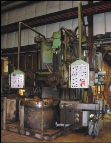
SCHIESS Vertical Turret Lathe , 52" cap., pendulum controls, dual head (1 head broken), 90 hp., s/n 32733404.
