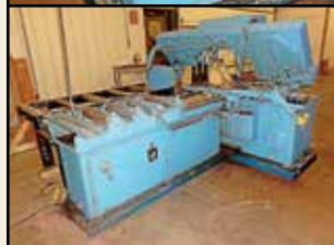
DoALL Horizontal Bandsaw , Mdl. C1216A, automatic power feed, 12" x 16" cap., VS, 85-450 FPM, 5 HP, 48" discharge table, 18" x 10' roller conveyor table, SN 423-84124, 1984.
