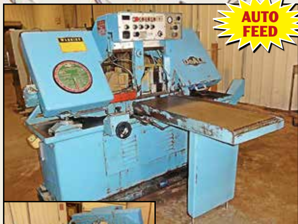
DoALL Horizontal Bandsaw , Mdl. C1216A, automatic power feed, 12" x 16" cap., VS, 85-450 FPM, 5 HP, 48" discharge table, 18" x 10' roller conveyor table, SN 423-84124, 1984.
