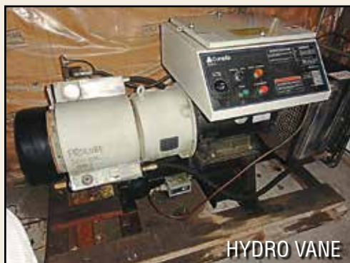
COMP AIR Hydro Vane Screw Compressor , Type 68 PAUS, 15 HP, 125 max. PSI, SN 068-000313/B, 41,937 hrs.
