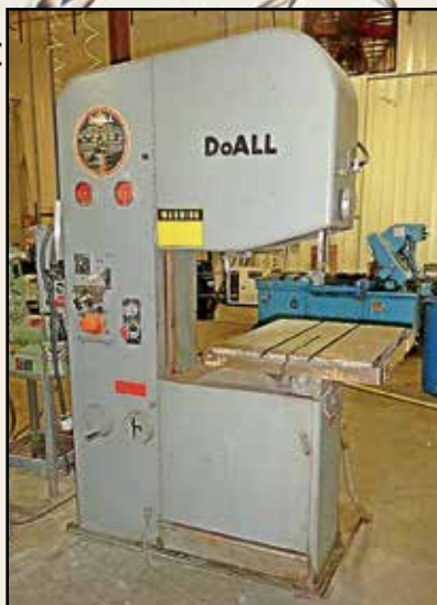
DoALL Vertical Bandsaw , Mdl. 2613-1H, 24" x 30" table, 14" under, 27" throat, w/blade welder, SN 361-79219, 1979.
