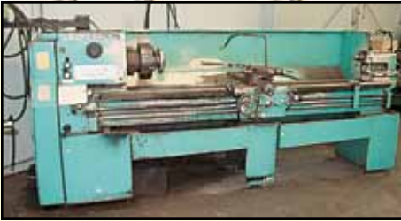
1985 LEBLOND Regal Lathe , 19" x 78", 12" 4-jaw chuck, TS, comp. cross slides, 10 hp, w/Mitutoyo 2-axis DRO, s/n 14F-326.
