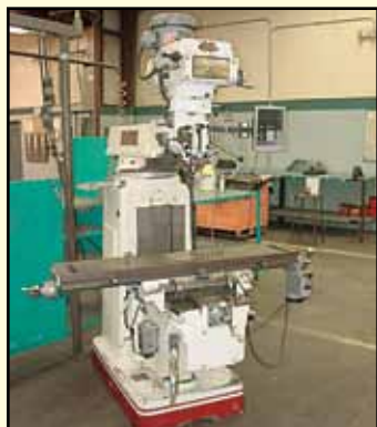
1993 ACER Vertical Mill, Mdl. 3VKH Ultima, 10" x 50" table, w/Newell C80 2-axis DRO, PF@X, s/n 9388233.
