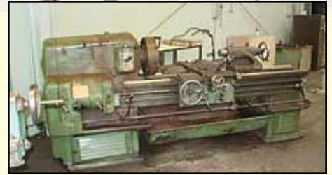
AMERICAN Lathe , Mdl. Pacemaker, 16" x 54", 15" 4-jaw chuck, TS, comp. cross slides, taper attach., s/n 73647-53.
