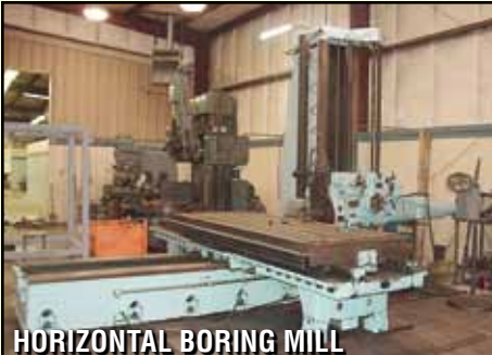
HORIZONTAL BORING MILL G & L Horizontal Boring Mill , Mdl. DT52, 48" x 122" table, 92" under, 5" spindle, Acra 130 3-axis DRO, X = 108", Y = 72", Z = 72".
