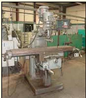
BRIDGEPORT Series II Vertical Mill, 11" x 58" table, VS, PF@X, Accurite 3-axis DRO, s/n 1495.
