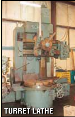
TURRET LATHE SCHIESS Vertical Turret Lathe , 39" table, 2-axis DRO, 5-station.
