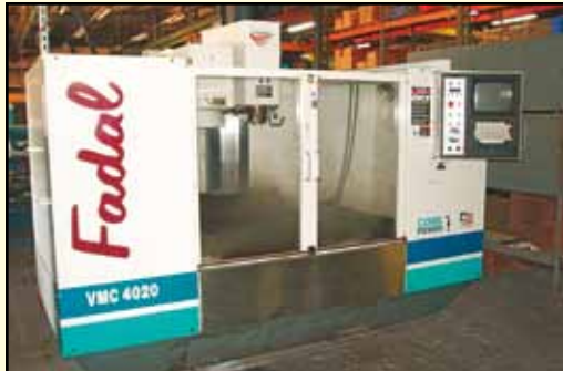
1998 FADAL VMC 4020HT Machining Center, Mdl. 906-1, X=40", Y and Z=20", Cat 40 taper, 21 ATC, 15 hp, 75-10,000 RPM, w/Fadal CNC 88HS control, s/n 9812170.
