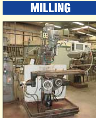
BRIDGEPORT CNC Vertical Mill, 9" x 48" table, VS, w/3-axis servo drive, s/n 277917E.
