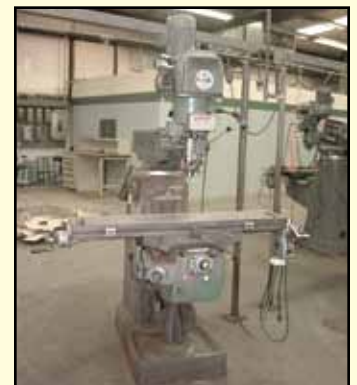
LAGUN Vertical Mill, Mdl. FT2, 9" x 48" table, w/Accurite III 2-Axis DRO, PF@X.
