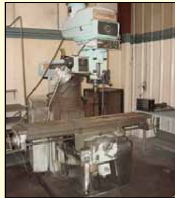
BRIDGEPORT Series II Special Vertical Mill, 11" x 58" table, w/Newell 2-axis DRO, PF@X, s/n 72859.
