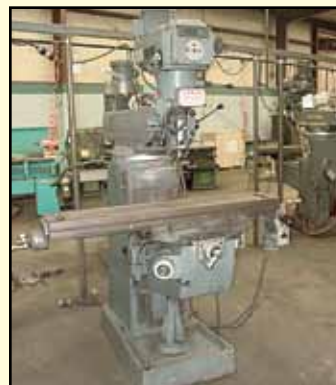
LAGUN Vertical Mill, 10" x 50" table, w/DRO, VS, PF@X.
