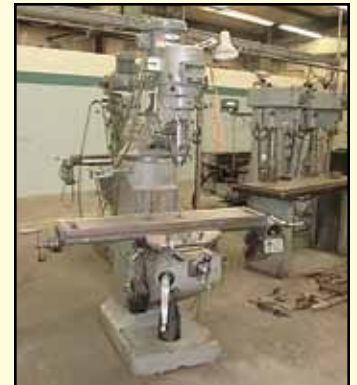
BRIDGEPORT Series I Vertical Mill, 9" x 48" table, w/Newell 2-axis DRO, VS, PF@X, s/n 270181.
