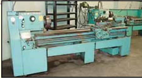
1977 LEBLOND Regal Lathe , 19" x 78", 12" 4-jaw chuck, TS, comp. cross slides, 10 hp, s/n 9F-579.
