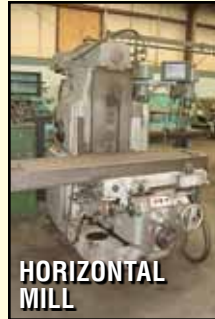
< HITACHI Horizontal Mill , Mdl. 3, 14" x 63" table, w/Newell Sapphire 2-axis DRO, s/n 713558-11.
