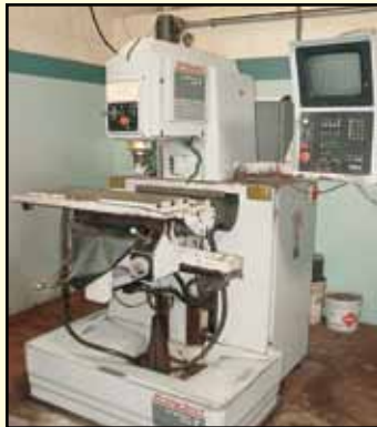
BRIDGEPORT CNC Mill, Mdl. Interact MK21, 12.5" x 34" table, w/BP Heidenhain TNC2500 control, s/n 665490890D.
