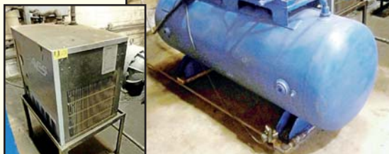
AES Air Dryer , Mdl. DHT-50, 50 SCFM, 200 max. PSI, 100 deg., SN HICES12219.
