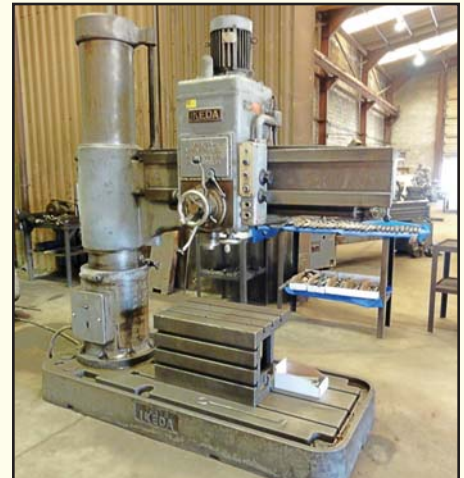
IKEDA Radial Arm Drill , Mdl. RM-1300, 4.5' arm, 13" column, 30–1,440 RPM, #5 Morse taper, quick disconnect tooling, 27" x 17" box table, 5 HP, SN 77067.
