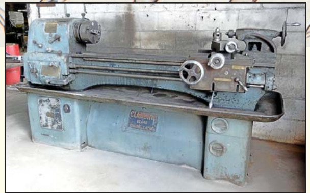
CLAUSING Colchester Geared-Head Lathe , Mdl. 6535, 15" swing x 48" centers, 2" spindle bore, 8" 3-jaw chuck, SN 311436.
