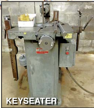
MORRISON Keyseater , Mdl. K, 1-1/4" cap., SN K702323 w/(3) cutter bars and tooling.
