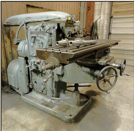
OHIO Horizontal Mill , #50 taper tooling, rapid travel, w/(2) heads (one Bridgeport type vertical head), 16.5' x 6' table w/tooling.
