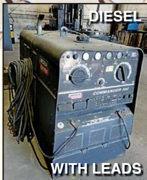
LINCOLN Commander 300 Diesel Welder/Generator , Mdl. K1525-2, SN U1990109215, 1,432 hrs.
