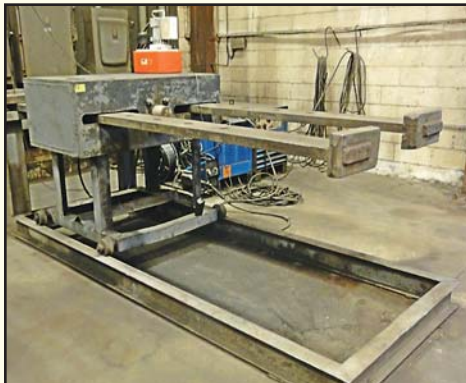
Horizontal Bulldozer Press , 100-ton cap., 6.5' vertical arm travels, 72" horizontal arm travel, 3" ram, w/adjustable head, w/OTC Series SS electric hydraulic pump.
