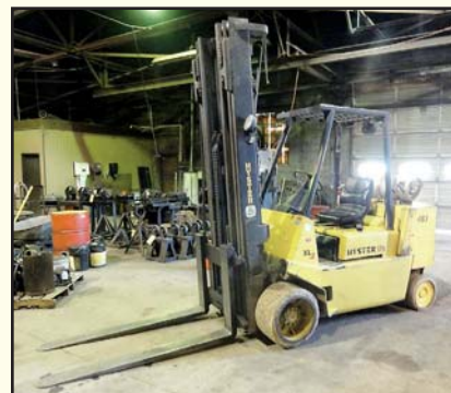
HYSTER 120 Forklift , Mdl. S120XL25, 6,500-lb. cap., 3-stage mast, LP gas, SN D004D104384.
