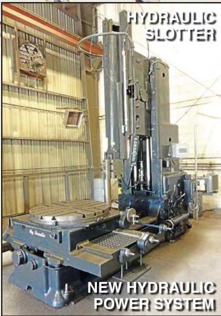
ROCKFORD Hydraulic Slotter , Mdl. SL, Series #3, 20" rating, 36" max. stroke, 6" min. stroke, 83" slots to center, 40" max. dist. under adj. ram guide, 0–10 deg. ram angle adj., 0–80"/min. cutting speed, 10,800-lb. max. cut pressure, 16" vertical adj. ram guide, 36" cross travel, 42" longitudinal travel, 0–140" range of cross feed and long. travel, 0–108" circular feed to table (on 12" circle), 42" rotary table dia., 20 HP, NEW Flow Dynamics and Automation 25 HP hydraulic unit – installed 2016 (for $30,000).
