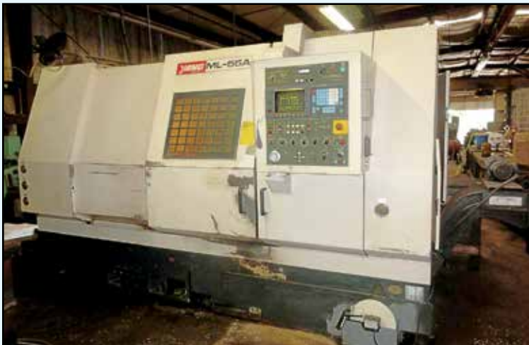
YANG Turning Center , Mdl. ML-55A, X=13.7", Z=43.3", 28.3" swing, 17.7" max. turn, 47.2" DBC, 15" 3-jaw chuck, 12-position turret, 2,000 RPM, Fanuc OT control, SN K10140.
