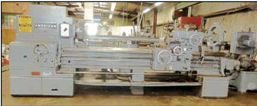
AMERICAN Lathe , Style D, 20" x 78", 20" swing over bed, 11.5" over cross slide, 78" DBC, 15" 4-jaw chuck, TS, w/tracer attachment, 2" hole, 25-1,500 RPM, SN 77305.
