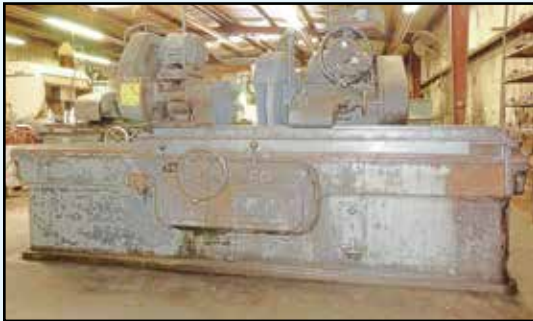
LANDIS Universal Grinder , 10" x 48", Accu-Rite II DRO.
