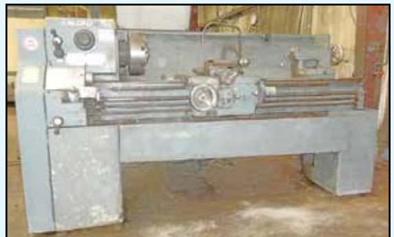
LeBLOND Regal Lathe , Mdl. X-2499, 15-1/2" swing over bed, 9-1/2" swing over cross slide, 30" DBC, 12" 4-jaw chuck, TS, taper attachment, 2-1/4" hole, 45-1,800 RPM, SN 11C-1221.
