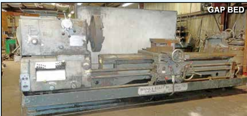
BINNS & BERRY TB Lathe Gap Bed Lathe , 30" x 115" bed, 20" swing over bed, 48" swing over gap, 92" DBC, 24" 4-jaw chuck, TS, 4" hole, SN UK.
