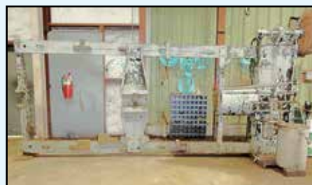
Wheel Press , 200-ton cap., 11' frame, hydraulic.
