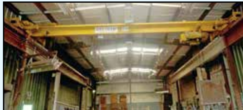
DIXIE Bridge Crane , 5-ton, Chandler Henry hoist, single-grinder, top running, under hung hoist, pendant control.
