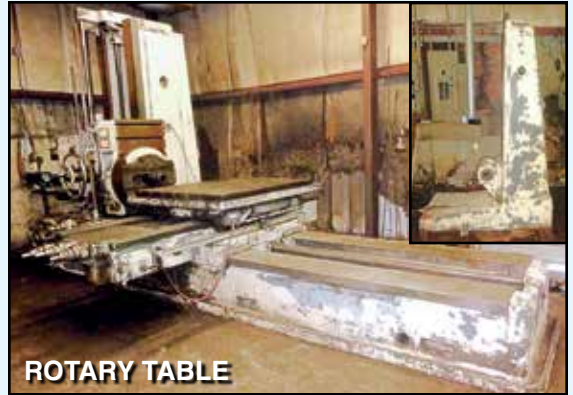
CERUTI Boring Mill , Mdl. AU110, 47-1/4" x 55-1/8" table, 16,500 max. table load, 4-21/64" spindle, #6 Morse taper, 27-speed from 2.5-1,000 RPM, 31-1/2" spindle travel, 49-1/8" spindle to table max. height, 56" vertical travel, 56" longitudinal travel, 63" cross travel, 27-9/16" face plate, 9-27/32" travel of facing slide, 157-1/2" max. dist. faceplate to SR, 2-axis DRO, w/tailstock, SN 10801.
