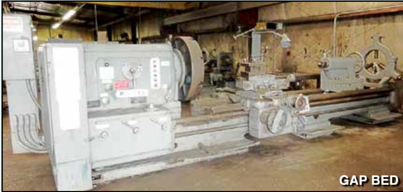
POREBA Gap Bed Lathe , Mdl. TR100 B1, 42" x 172.5" bed, 40" swing over bed, 26.77" swing over cross slide, 49.25" swing @ gap, 120" DBC, 31.5" 4-jaw chuck, tool post, TS, SR, 4-3/4" hole, taper attachment, DRO, SN 1191-181.
